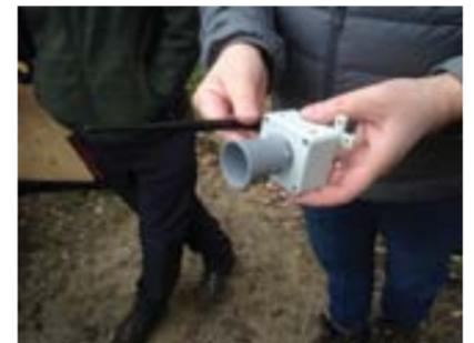
Ultrasonic river monitoring device suspended from bridge soffits at Hardcastle Craggs.
